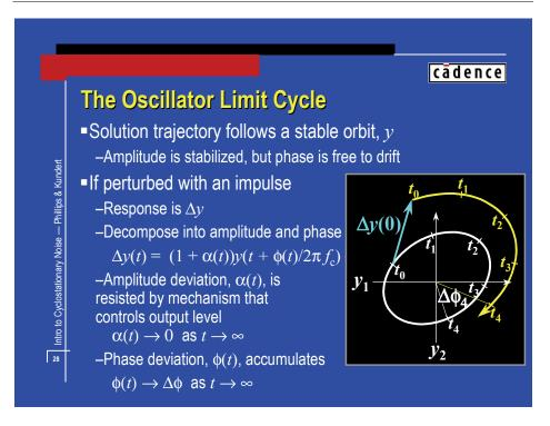
Consider plotting the capacitor voltage against the inductor current in a resonant oscillator. In steady state, the trajectory is a stable limit cycle. Now consider perturbing the oscillator with an impulse  $x = \delta(t)$  and assume that the response to the perturbation is  $\Delta y$ . Separate  $\Delta y$  into amplitude and phase variations,
