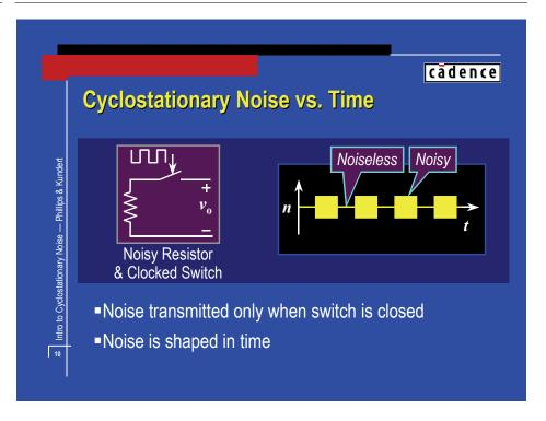
This is a simple example of cyclostationary noise. A periodically operating switch between the noise source (the resistor produces white thermal noise) and the observer causes the output noise to vary periodically.
