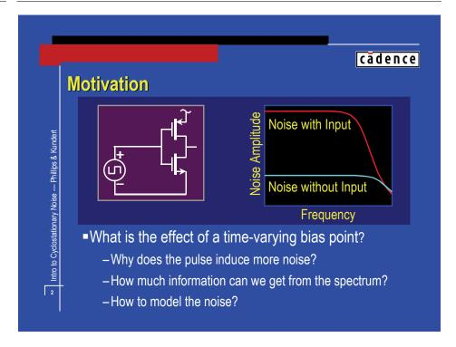
SPICE noise analysis is not able to compute valid noise results for many common classes of circuit for which noise is of interest. Noise in these circuits is of different character than that can be computed by SPICE. We show why and how in this presentation. We explain how this noise differs from the noise discussed in introductory text books on noise, and how this difference affect your circuits.
