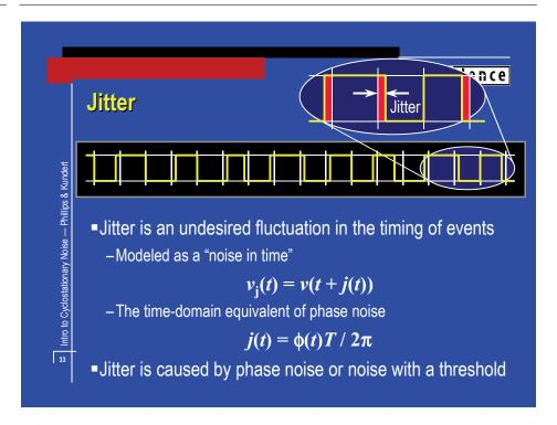
Jitter is an undesired fluctuation in the timing of events. It can be modeled as a noise in time. It is equivalent to phase noise and is used in situations where it is more natural think of the noise being in time rather than in phase or in signal level. Like phase noise, it serves to degrade system performance.
