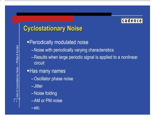
Though the term *cyclostationary noise* may be unfamiliar, it is critically important to most designers. They typically know it by other names: oscillator phase noise, jitter, noise folding, AM & PM noise, etc. By looking at noise using the common theoretical foundation of cyclostationary noise allows designers to better understand and predict all of these manifestations of noise.
