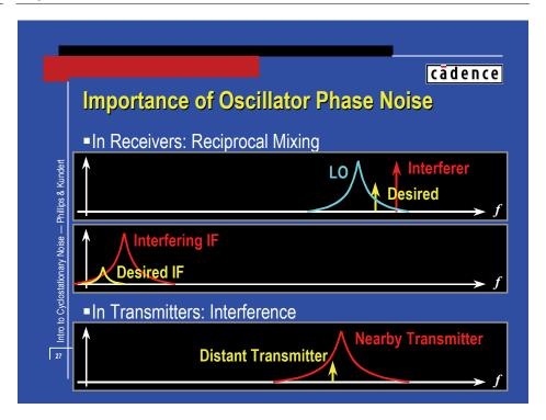
In a receiver, the phase noise of the LO can mix with a large interfering signal from a neighboring channel and swamp out the signal from the desired channel even though most of the power in the interfering IF is removed by the IF filter. This process is referred to as *reciprocal mixing*.
