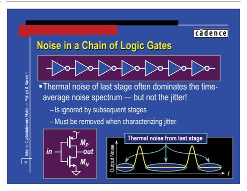
The total output noise power of a gate is dominated by the thermal noise produced by the output devices if the gate spends most of its time with an unchanging output. This noise is usually ignored by subsequent stages. Thus, using the time-averaged spectral density to characterize the noise in a gate is misleading. Only the noise produced by a gate at the point where its output crosses the threshold of the subsequent stage should be taken into account when characterizing the jitter of the gate.
