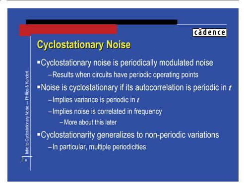
Cyclostationary noise results when noise is periodically modulated. This occurs in any nonlinear circuit that is driven by, or exhibits, large periodic signals.
