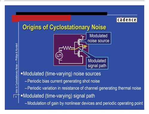
Cyclostationary noise is generated by circuits with periodic operating points. The timevarying operating point modulates the noise generated by bias-dependent noise sources, and modulates the transfer function from the noise source to the output. Both result in cyclostationary noise at the output.
