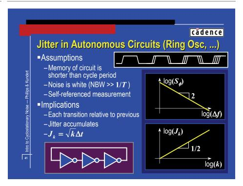
Next, consider a simple autonomous circuit such as an ring oscillator. Assume that the noise sources in the circuit are all white and that  $J_k$  is measured using a self-referred measurement. In this case, the jitter variance accumulates from cycle-to-cycle, and so  $J_k = k^{1/2} \Delta t$ .
