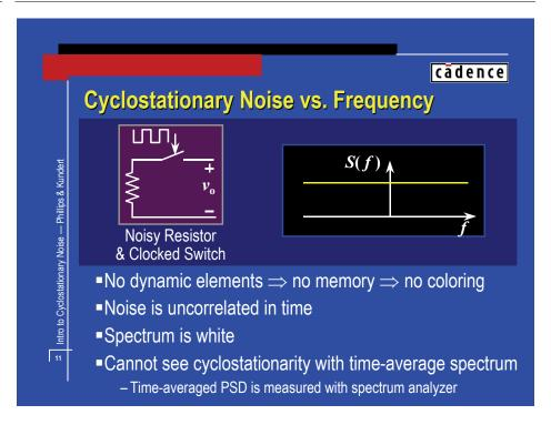
With no energy storage elements the noise is completely uncorrelated (noise at a particular time is uncorrelated with the noise at any previous time) and therefore is white, even though it is cyclostationary. One cannot tell that noise is cyclostationary by just observing a simple PSD.
