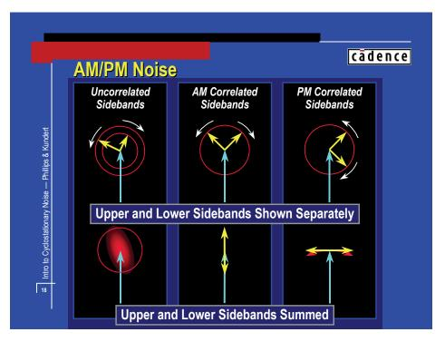
With cyclostationary noise, the noise in various sidebands is correlated. Depending on the magnitude and phase of the correlation, the noise at the output of the circuit can be AM noise, PM noise, or some combination of the two. For example, oscillators almost exclusively generate PM noise near the carrier whereas noise on the control input to a variable gain amplifier results almost completely in AM noise at the output of the amplifier.
