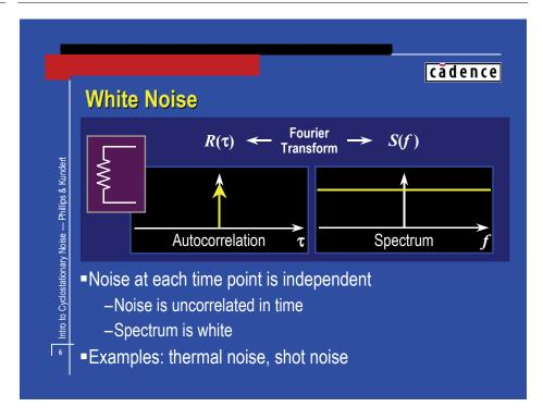
There are two ways of characterizing noise, the power spectral density or PSD, S(f), and the autocorrelation function,  $R(t,\tau)$ . These two representations are related by the Fourier transform.
