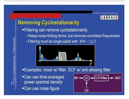
If a stage that generates cyclostationary noise is followed by a filter whose passband is constrained to a single sideband (the passband does not contain a harmonic and has a bandwidth of less than  $f_0/2$ , where  $f_0$  is the fundamental frequency of the cyclostationarity), then the output of the filter will be stationary. This is true because noise at any frequency  $f_1$  is uncorrelated with noise at any other frequency  $f_2$  as long as both  $f_1$  and  $f_2$  are within the passband.
