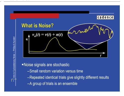
Noise free systems are deterministic, meaning that repeating the same experiment produces the same result. Noisy systems are stochastic — repeating the same experiment produces slightly different results each time. An experiment is referred to as a trial. A group of experiments is referred to as an ensemble of trials, or simply an ensemble.
