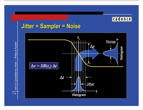
Jitter in the time at which a signal is sampled creates noise in the sampled result if the signal is changing at the time it is sampled. This is one way in which noise is generated when converting continuous-time signals are converted to discrete-time signals. The statistics of the noise can be computed from the statistics of the jitter at the time of the sampling and the slewrate (or time derivative) of the input signal at the time of the sampling.
