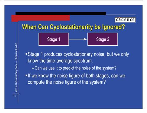
Sometimes it is only possible to determine the time-average PSD. So an important question is, when is it good enough? In other words, if you have a stage that is producing cyclostationary noise that drives another stage, and you know the time-average spectrum of the noise produced by the first stage, when is that enough to allow you to predict the effect of that noise on the subsequent stage.
