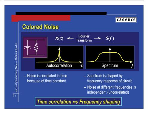
Energy storage elements cause the circuit to exhibit a frequency response that is shaped; it is not flat with frequency. As such, it causes the PSD to be shaped. This is referred to as coloring the noise. Colored noise has a PSD that varies with frequency.
