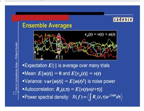
Assume that  $v_n(t) = v(t) + n(t)$ , where v(t) is the deterministic signal, n(t) is the noise, and  $v_n(t)$  is the combined signal.
