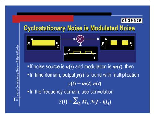
As mentioned before, cyclostationary noise is another name for modulated noise. Cyclostationary noise can be created by periodically modulating stationary noise. Similarly, cyclostationary noise can always be decomposed into, or modeled as, a stationary noise and a periodic modulation.
