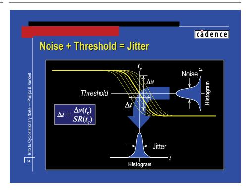
Noise added to a signal transitioning through a threshold adds jitter to the time at which the signal crosses the threshold. This is the way jitter is created in nonlinear circuits such as digital circuitry. The statistics of the jitter can be computed from the statistics of the noise at the time of the threshold crossing and the slewrate (or time derivative) of the large signal at the threshold crossing.
