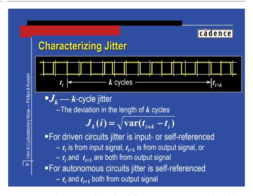
A common way to characterize jitter is k-cycle jitter,  $J_k$ . It represents the variation in the length of k cycles. If there is no jitter, then  $J_k$  will be 0, if the jitter on each cycle is completely uncorrelated with the jitter on previous cycles, then  $J_k$  will be constant with k, and if the jitter is correlated from cycle-to-cycle, then  $J_k$  will vary as a function of k.
