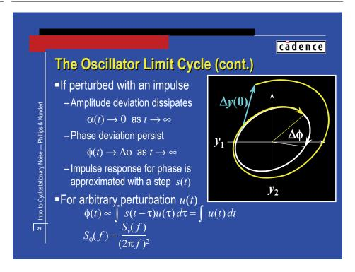
On the previous slide it was pointed out that  $\alpha(t) \to 0$  as  $t \to \infty$  and  $\phi(t) \to \Delta \phi$  as  $t \to \infty$ . If we neglect any short term time constants, it can be inferred that the impulse response of the phase deviation  $\phi(t)$  can be approximated with a unit step s(t). The phase shift over time for an arbitrary input disturbance u is
