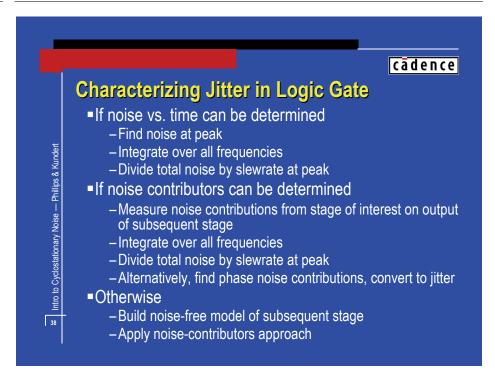
There are several different methods that can be used to determine the jitter of a logic block using a simulator such as SpectreRF. They all assume that the circuit is driven, so as to produce a periodic response, and that a cyclostationary noise analysis is performed about that periodic operating point.
